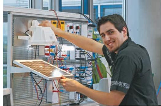
knowledge on photovoltaics in a practical manner and the solar energy lab is used to train future photovoltaics professionals. The training system heat pump with solar thermal energy and photovoltaics consists of six training booths that can be combined in varying manner depending on the training target. This allows for the setting up of different facility concepts, to assess them metrologically and evaluate them in comparison to each other.
